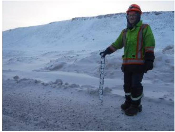
Photo 12 Snow bank heights measured from the road surface up to the top of the bank on both the east and west banks at set locations, February 6, 2018.
