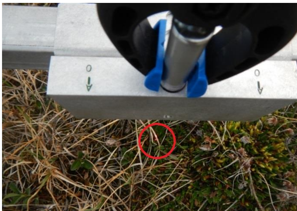
Photo 5 A view showing the diameter of the laser projecting onto the vegetation (2 mm), 27 July 2014.
