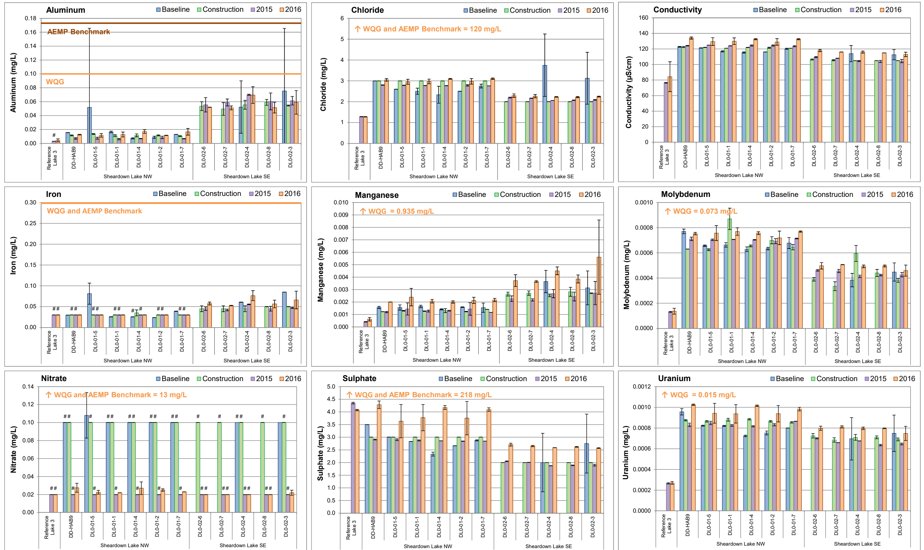
Figure 4.9: Temporal comparison of water chemistry at Sheardown Lake Northwest (DLO-01) and Sheardown Lake Southeast (DLO-02) for mine baseline (2005 - 2013), construction (2014), and operational (2015, 2016) periods during fall. Values represent mean \pm SD. Pound symbol (#) indicates parameter concentration is below the laboratory method detection limit. See Table 2.3 for information regarding Water Quality Guideline (WQG) criteria. AEMP Benchmarks are specific to Sheardown Lake (northwest and southeast).
