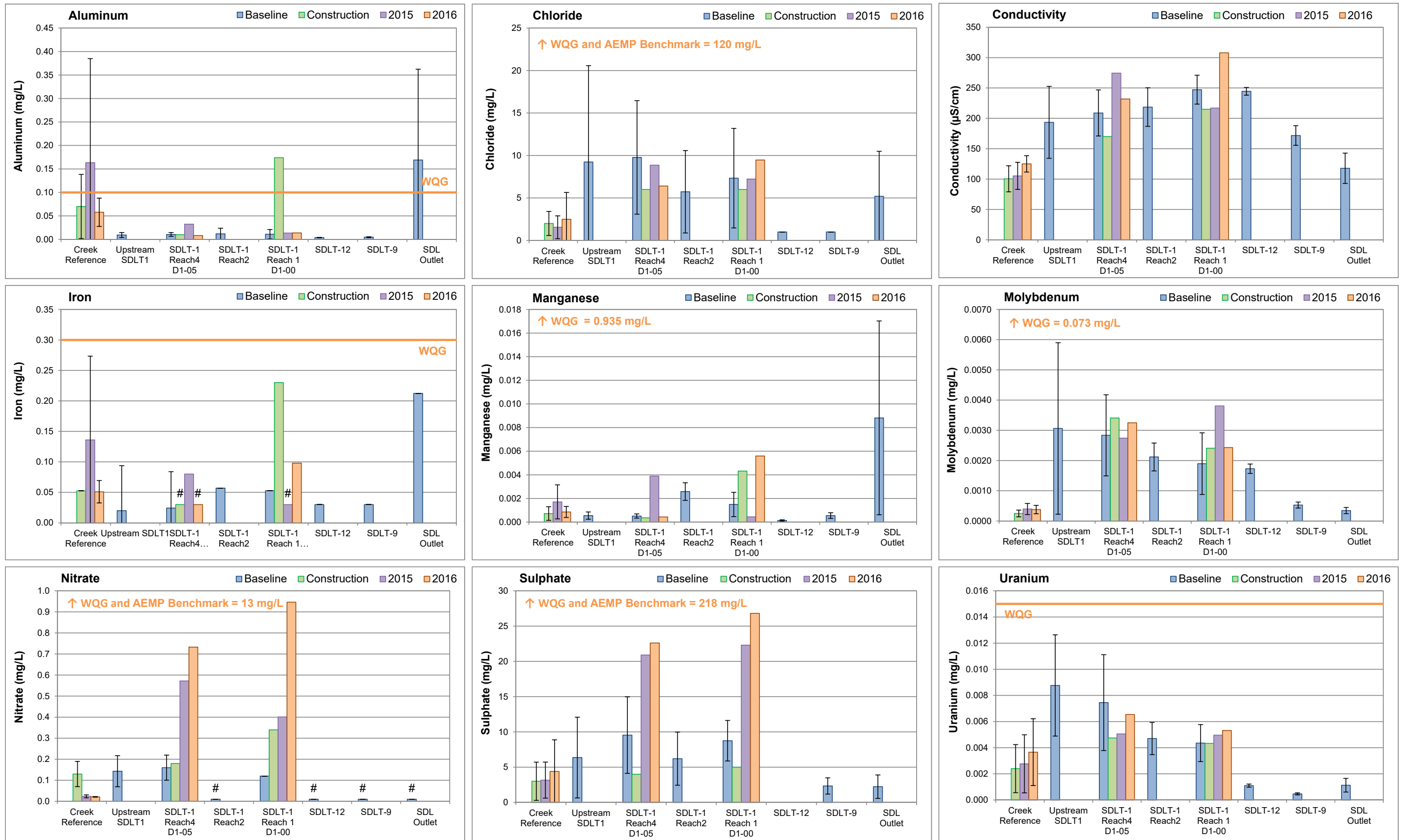
Figure 4.2: Temporal comparison of water chemistry at Sheardown Lake Tributaries (SDLT) for mine baseline (2005 - 2013), construction (2014) and operational (2015, 2016) periods during fall. Values represent mean \pm SD. Creek reference stations include the CLT-REF and MRY-REF series (mean \pm SD; n = 4). Pound symbol (#) indicates parameter concentration is below the laboratory method detection limit. See Table 2.3 for information regarding Water Quality Guideline (WQG) criteria. AEMP Benchmarks are adopted from the Camp Lake Tributaries.
