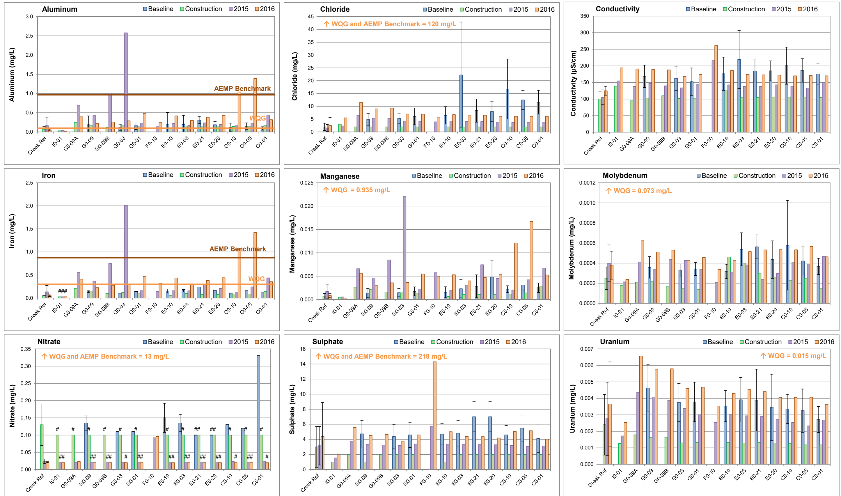
Figure 5.2: Temporal comparison of water chemistry at Mary River stations for mine baseline (2005 - 2013), construction (2014) and operational (2015, 2016) periods during fall. Values represent mean \pm SD. Creek reference includes CLT-REF and MRY-REF series stations (mean \pm SD; n = 4). Pound symbol (#) indicates parameter concentration is below the laboratory method detection limit. See Table 2.2 for information regarding Water Quality Guideline (WQG) criteria. AEMP Benchmarks are specific to Mary River.
