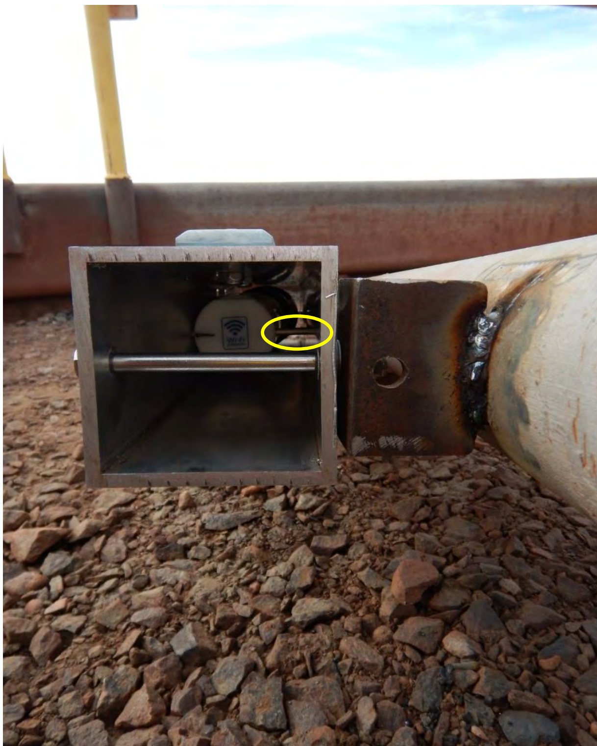
Figure 6 : Hardware attaching aluminum tube to L brackets and view of the primary tide gauge mounted in the tube. Yellow oval shows location of the 1/4" bolt that should pass through the end cap of the primary RBRconcerto 3 tide gauge.
