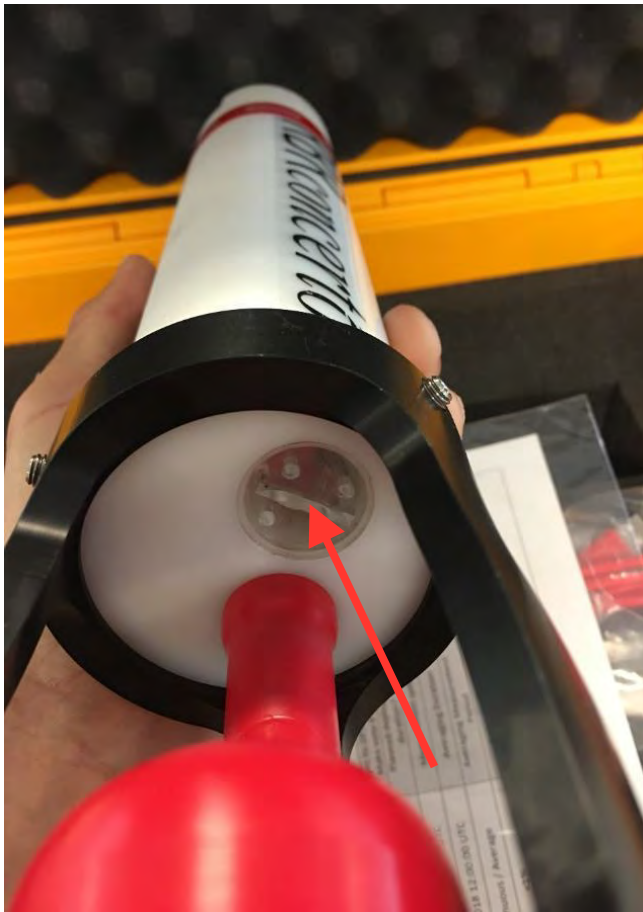
Figure 9: Pressure sensor location, shown by the arrow, on the downward facing end of the primary RBRconcerto 3 tide gauge
