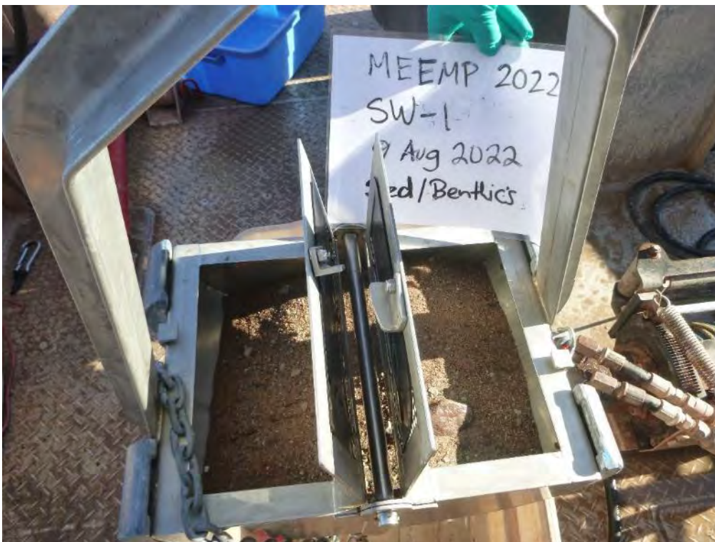
Photo 2 – Sediment sample collected in the Van Veen grab at station SW-1 on 09 August 2022.
