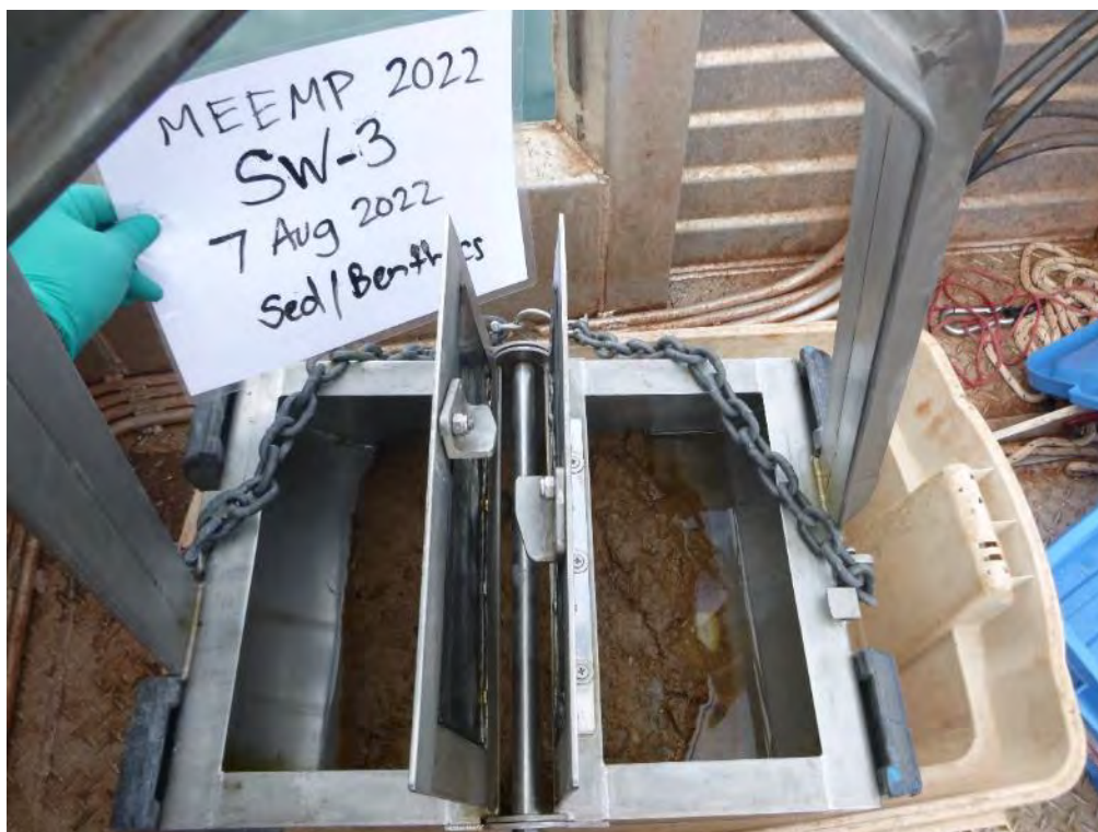
Photo 8 – Sediment sample collected in the Van Veen grab at station SW-3 on 07 August 2022.
