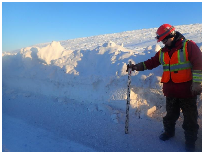
Photo 10-6. View of a non-compliant (140 cm) snowbank. Height management may be unsafe if terrain features limit machinery movement (km 55.8.0; February 11, 2020).
