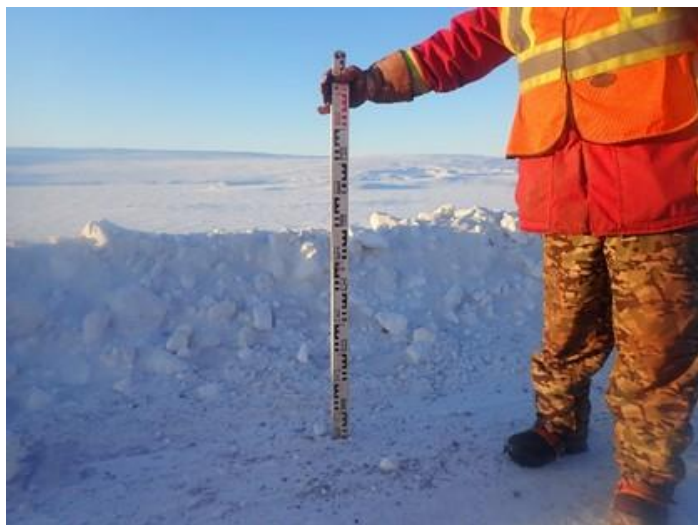
Photo 10-5. View of a compliant (60 cm) snowbank. Heights are measured from the road surface up to the bank's top at randomized locations along the Tote Road (km 56.0; February 11, 2020).
