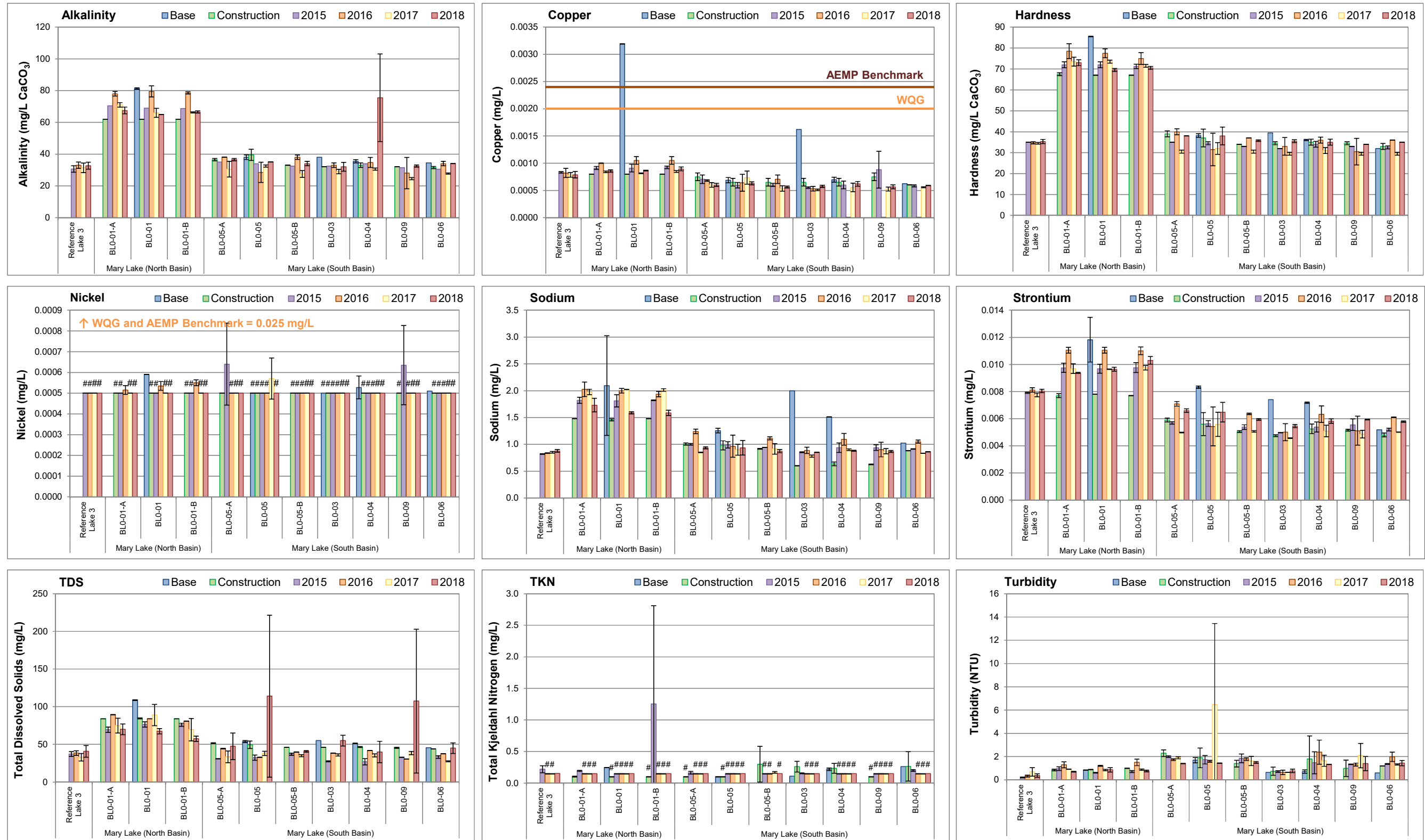
Figure C.28: Temporal Comparison of Water Chemistry at Mary Lake (BLO) for Mine Baseline (2005 to 2013), Construction (2014), and Operational (2015 to 2018) Periods during Fall
