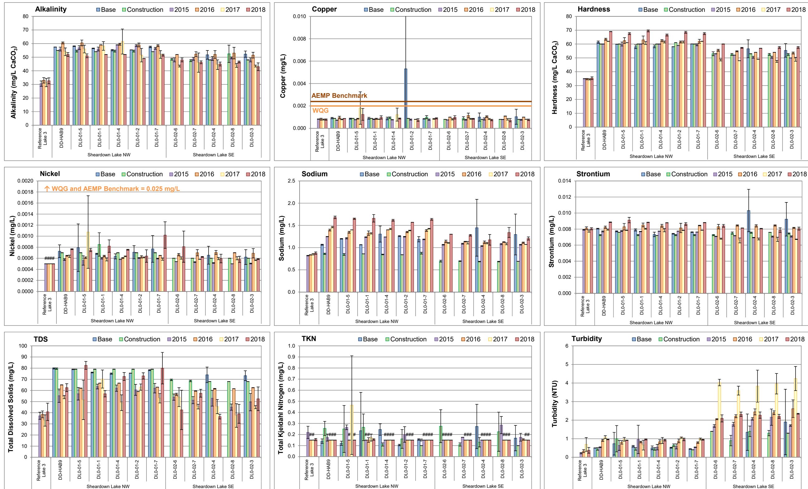
Figure C.19: Temporal Comparison of Water Chemistry at Sheardown Lake Northwest (DLO-01) and Sheardown Lake Southeast (DLO-02) for Mine Baseline (2005 to 2013), Construction (2014), and Operational (2015 to 2018) Periods during Fall
