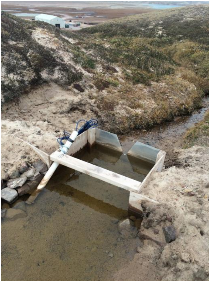
PHOTO 10 - Hydrology Monitoring Station Weir and Sensor, September 2016
