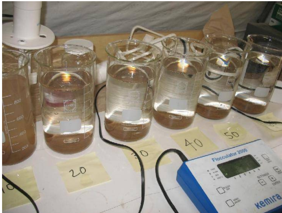
Photo 5 – Laboratory testing for flocculant dosing optimization.
