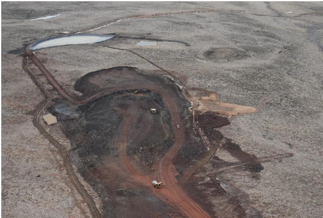
PHOTO 6 - Mary River Mine Site Waste Rock Stockpile and Waste Rock Sedimentation Pond, July 2016
