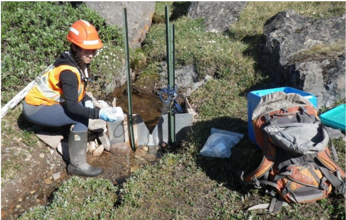
PHOTO 16 – Weekly Water Sampling at MQ-C-A with a Hydrological Monitoring Weir, July 2016
