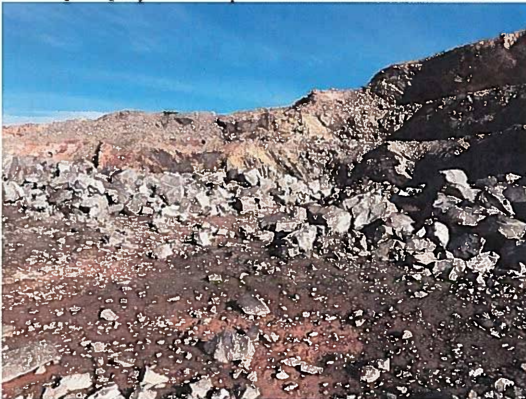
Photo 8: QMR2 Quarry. Much loose present of faces and bench width less than 8m
