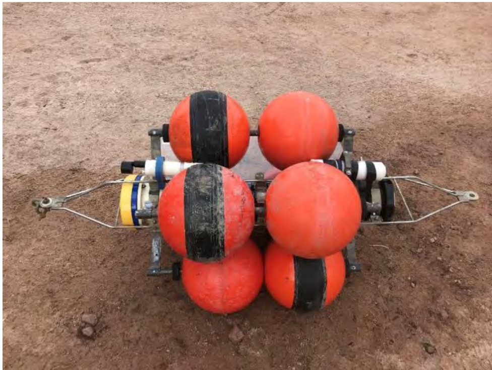
Photo 1 – Golder Bruce Head mooring with an up-looking Nortek Signature 500 kHz ADCP, a down-looking TRDI Sentinel Workhorse 300 kHz ADCP, an RBR CTD, and a XEOS Kilo Iridium beacon deployed in August 2019
