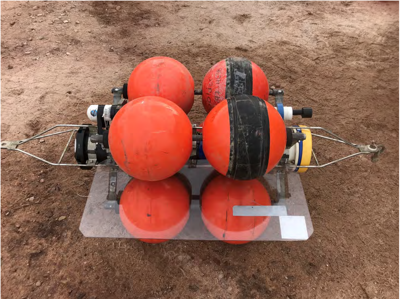
Figure 6: Bruce Head subsurface tautline mooring prior depicting the up-looking Nortek Signature 500 kHz ADCP, down-looking TRDI 300 kHz ADCP, RBR CT, satellite beacon, and Plexiglas fin
