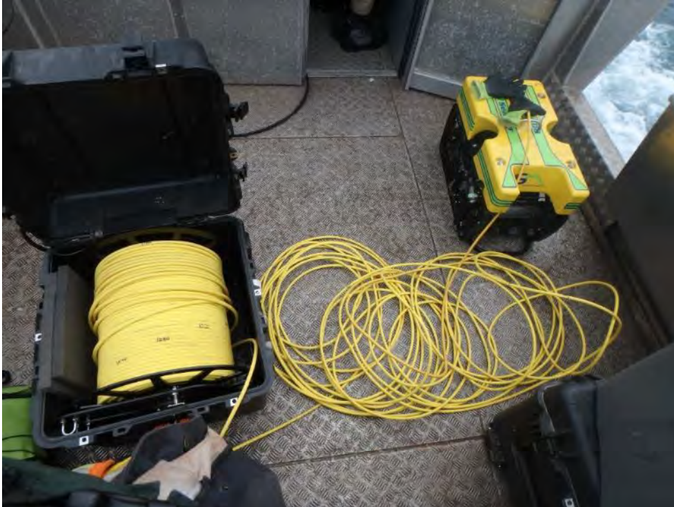
Photo 29 - Seamor Chinook 300F ROV video system used to undertake underwater video surveys of offset habitat along Milne Port Ore Dock in August 2019
