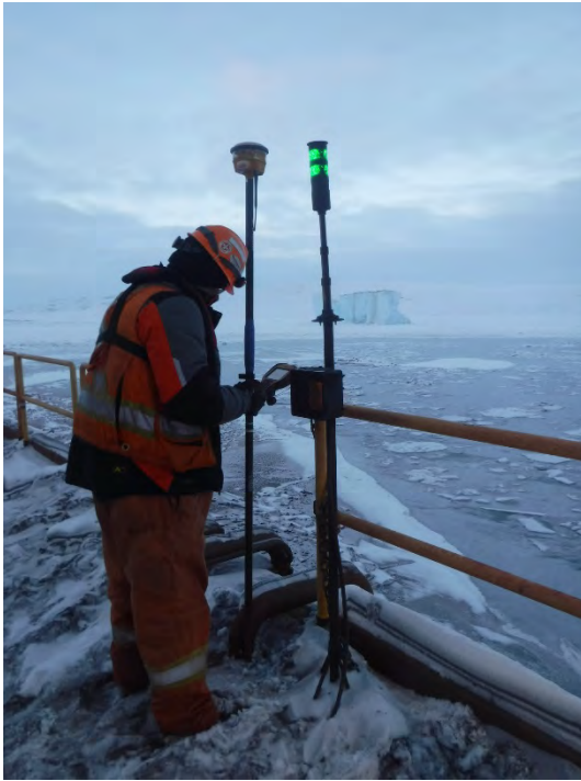
Figure 7: RTK GPS survey conducted in 2018
