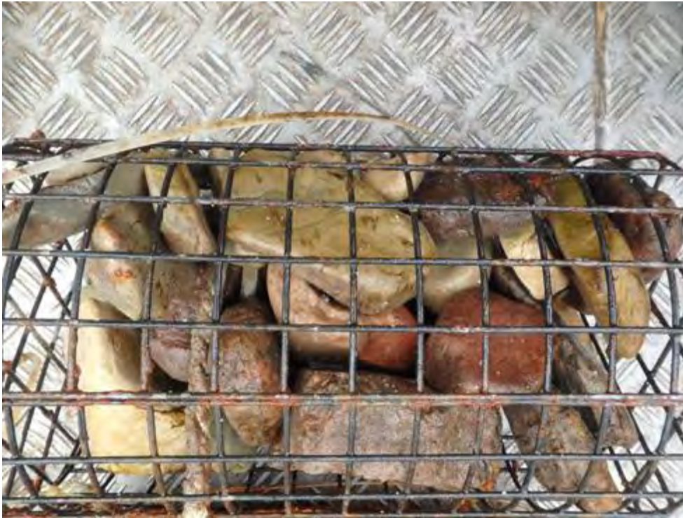
Photo 27 - Settlement basket (SBEO-1) retrieved from eastern side of the Milne Port Ore Dock in August 2019
