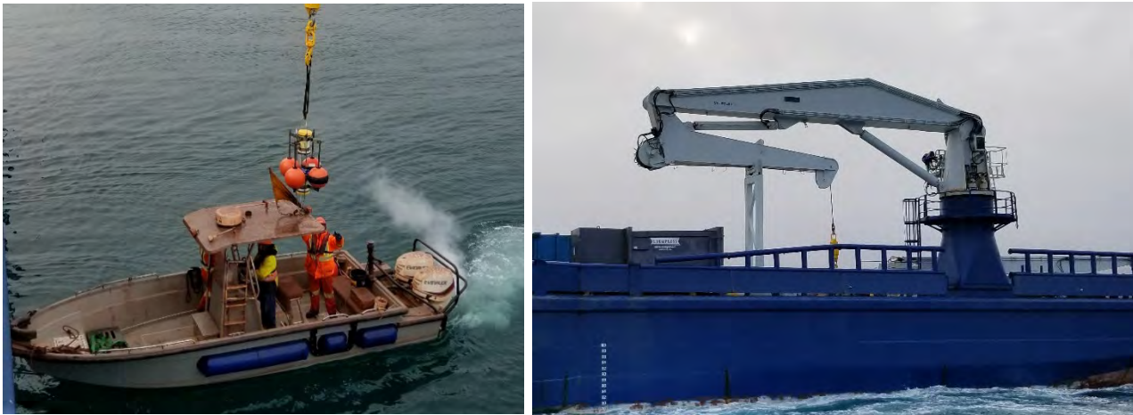
Figure 8: Milne Port 01 mooring being loaded onto tender vessel following recovery (left) and the Botnica port-side crane used for lifting moorings onto deck (right)
