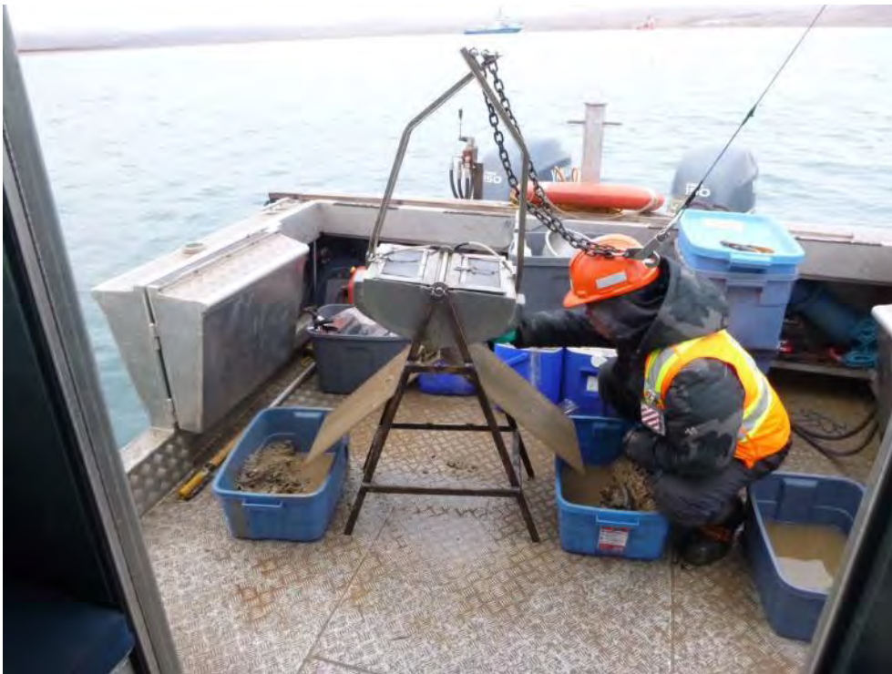
Photo 6 - A-frame field splitter being used to split a benthic sample collected using the Van Veen grab sampler
