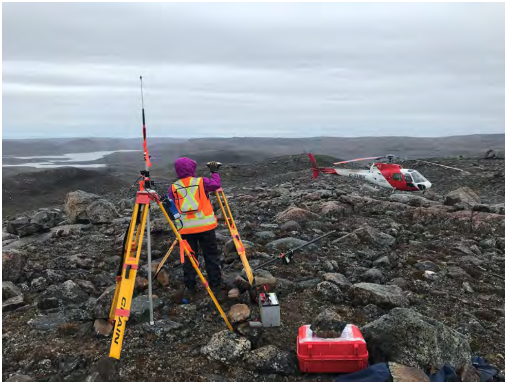
PHOTO 1 – Survey Lead Setting Up Base Station Prior to a Day of Legal Boundary Surveying at Eqe Bay
