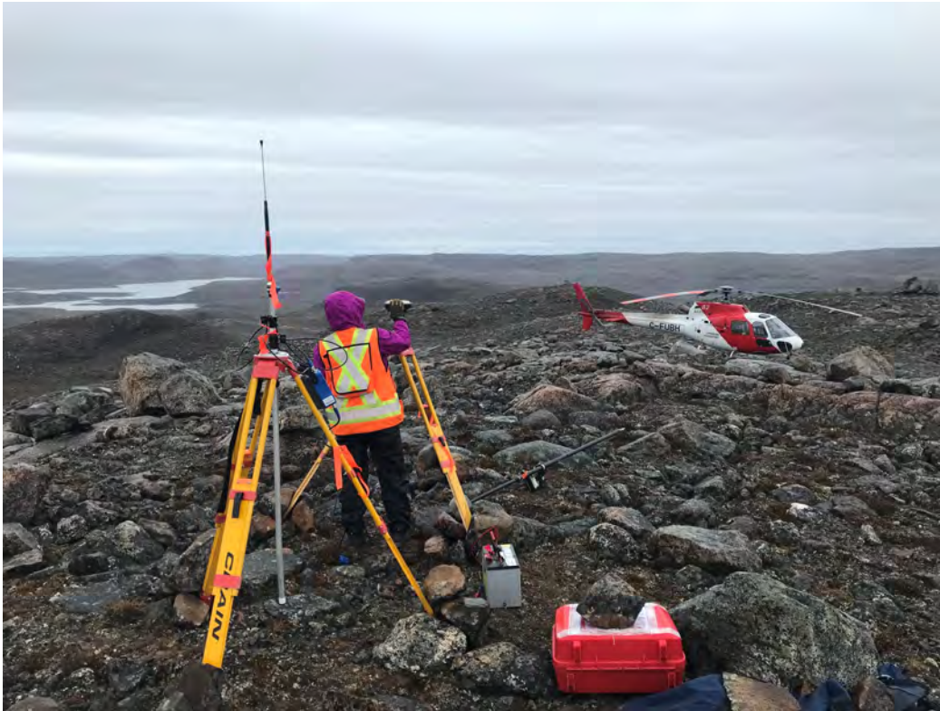
PHOTO 1 – Survey Lead Setting Up Base Station Prior to a Day of Legal Boundary Surveying at Ege Bay
