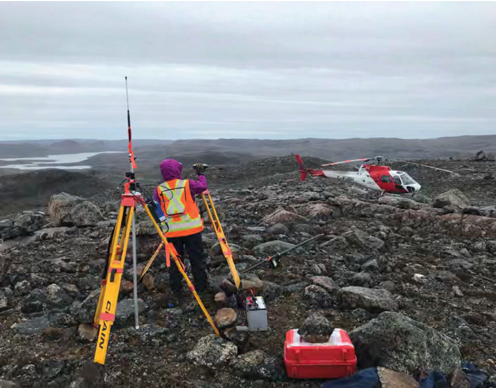
Survey Lead Setting up Base Station Prior to a Day of Legal Boundary Surveying at Ege Bay
