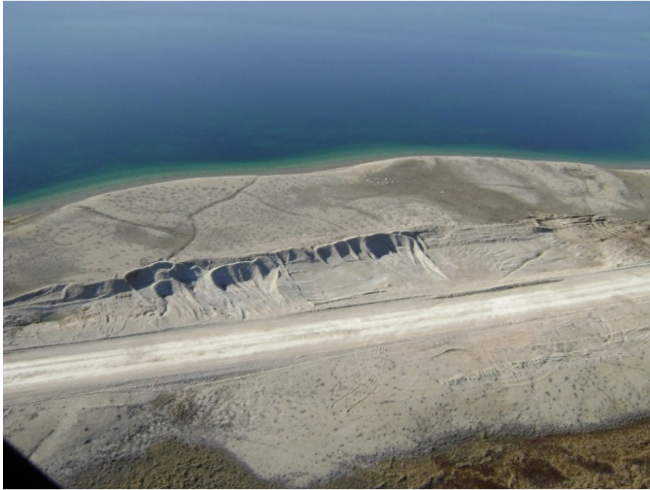
Photo 6 (2014 Photo 1576): Pit at KM 32.4 (Figures 4 and 5), typical Priority C pit in thaw stable soils that only requires regrading.
