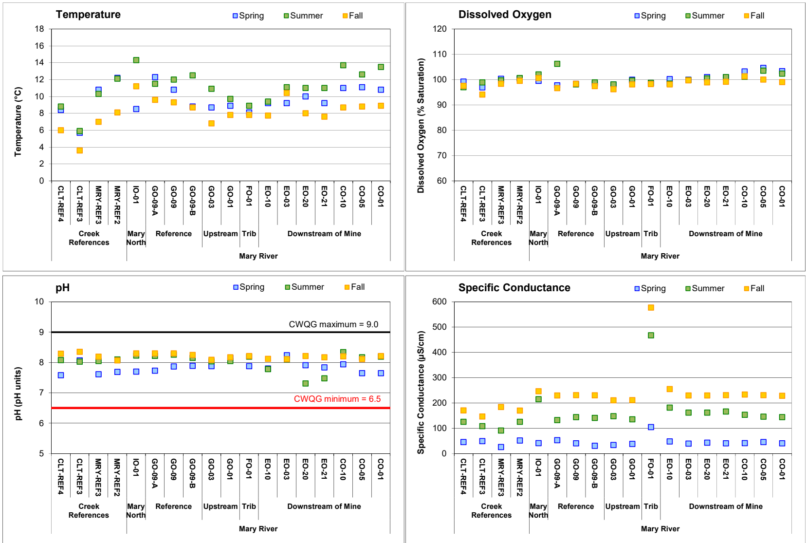
Figure 5.1: Comparison of In Situ Water Quality Variables Measured at Mary River Water Quality Monitoring Stations in Spring, Summer, and Fall 2019, Mary River Project CREMP
