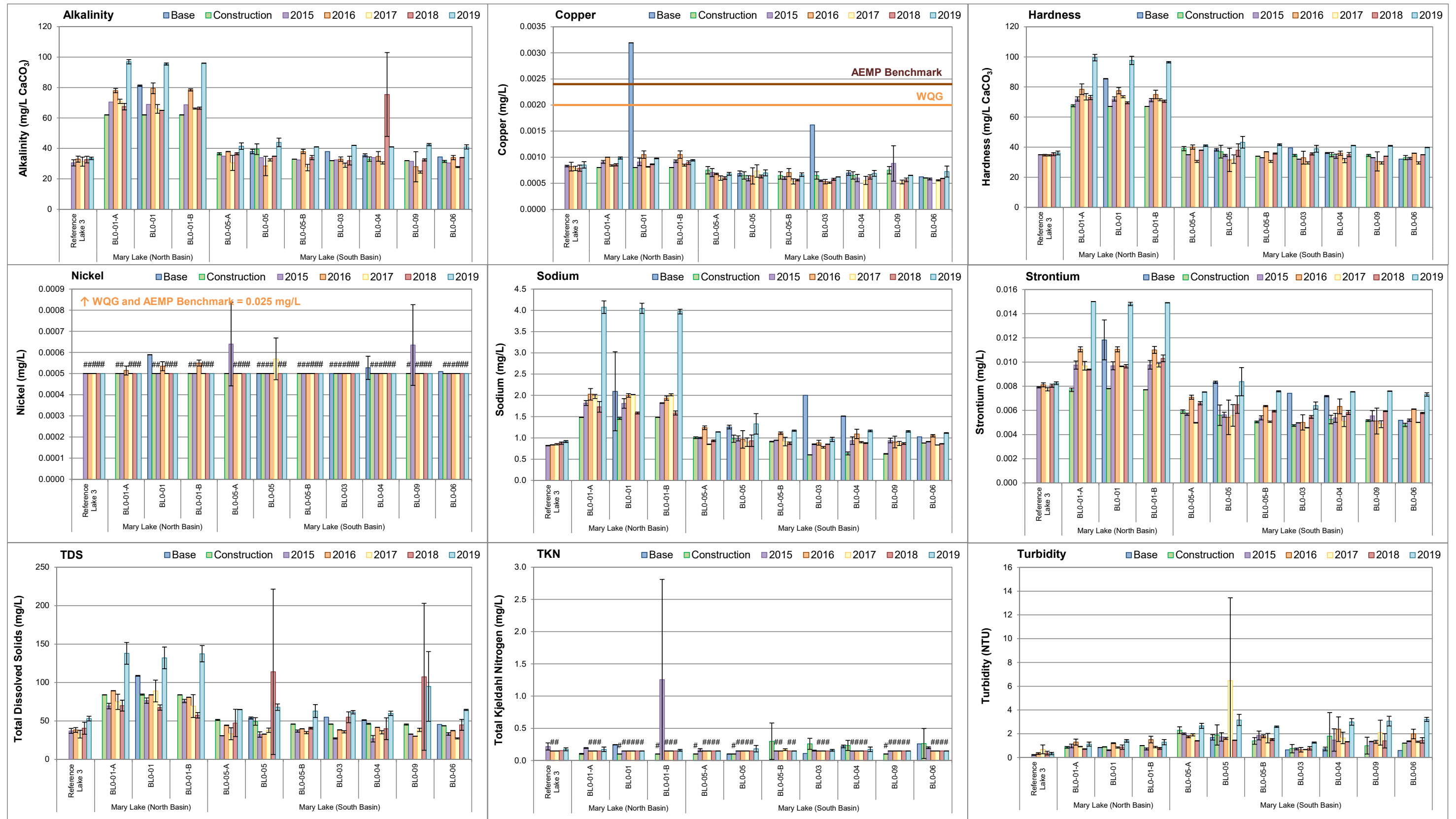
Figure C.27: Temporal Comparison of Water Chemistry at Mary Lake (BLO) for Mine Baseline (2005 to 2013), Construction (2014), and Operational (2015 to 2019) Periods during Fall
