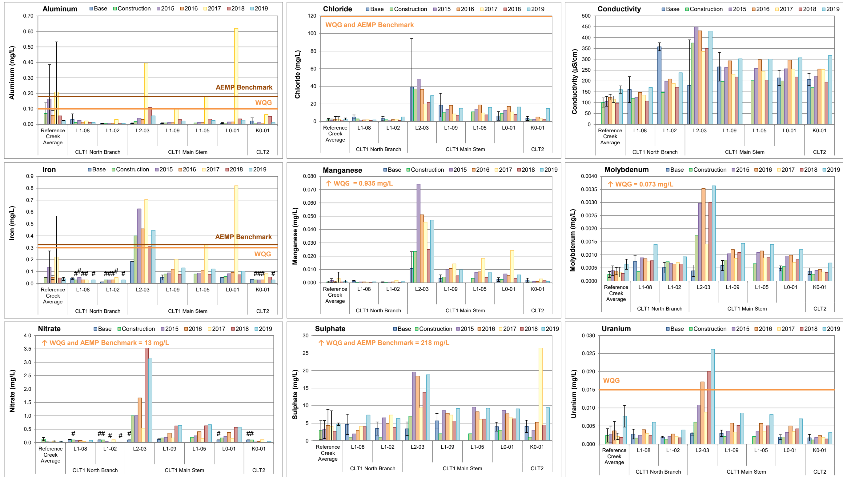
Figure 3.2: Temporal Comparison of Water Chemistry at Camp Lake Tributary 1 (CLT-1) and Tributary 2 (CLT-2) for Mine Baseline (2005 to 2013), Construction (2014) and Operational (2015 to 2019) Periods During Fall
