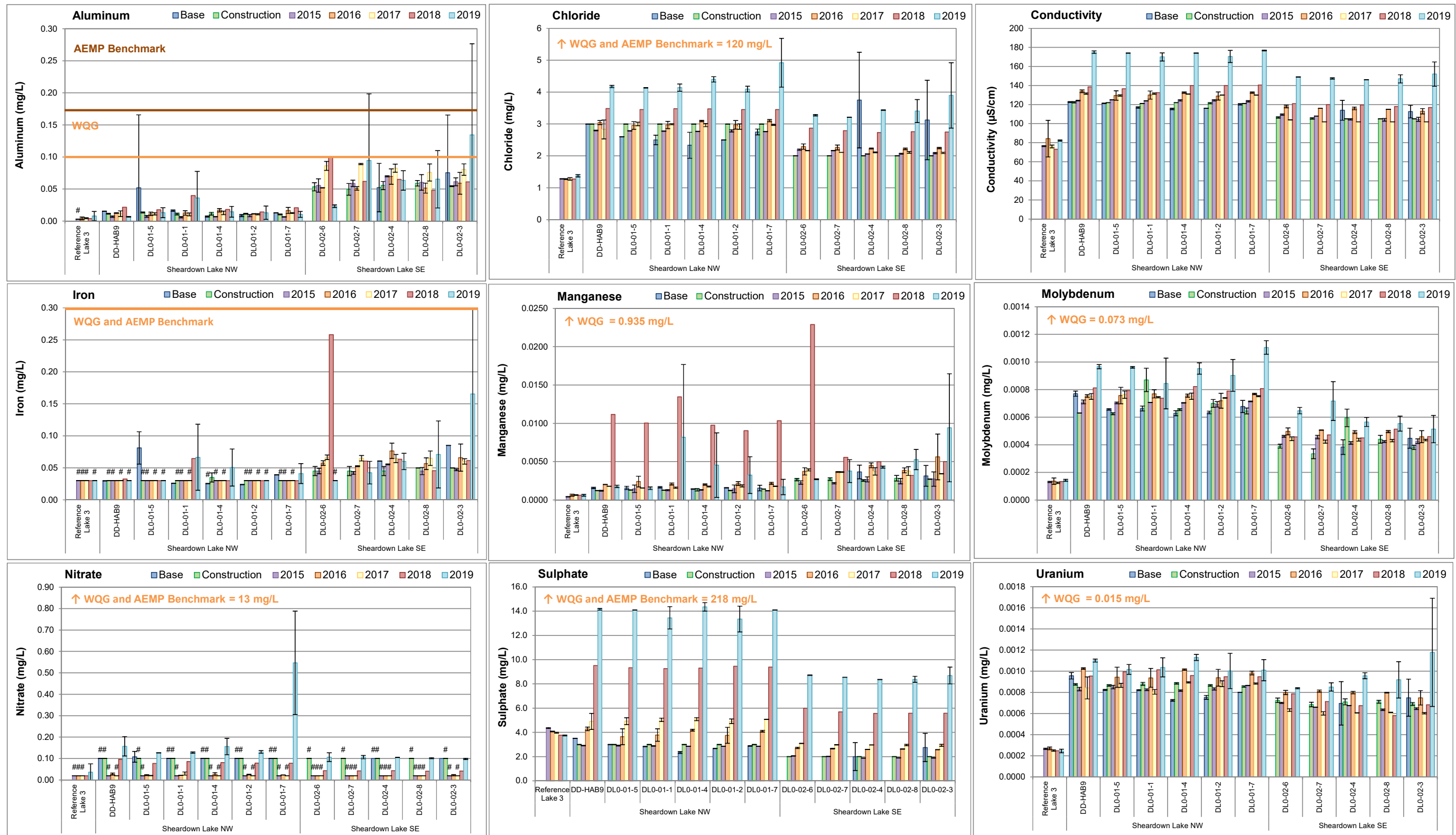
Figure 4.9: Temporal Comparison of Water Chemistry at Sheardown Lake Northwest (DLO-01) and Sheardown Lake Southeast (DLO-02) for Mine Baseline (2005 to 2013), Construction (2014), and Operational (2015 to 2019) Periods during Fall
